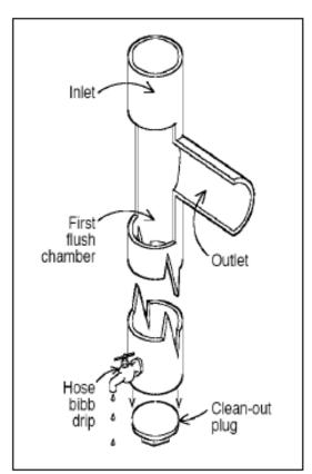
Figure 4.25. Diagram of a first flush diverter (photo: Texas Water Development Board, 2005).
