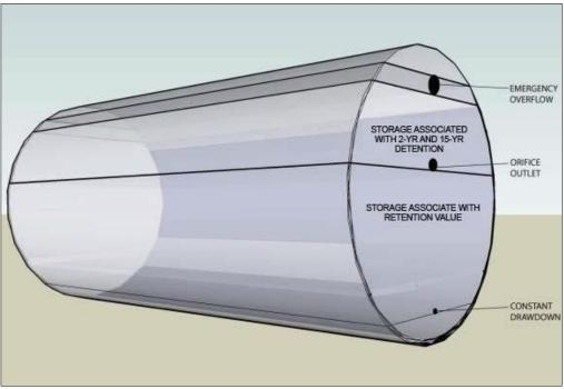
Figure 4.29. Cistern Design 3: Constant drawdown version where storage is associated with design storm, channel protection, and flood volume.
