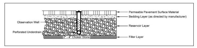
Figure 4.12. Cross-section of a standard permeable pavement design.
