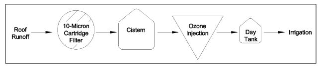
Figure 1. Example 1 treatment schematic.
