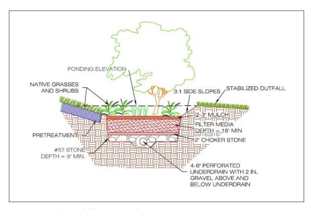
Figure 4.4. Example standard bioretention design.
