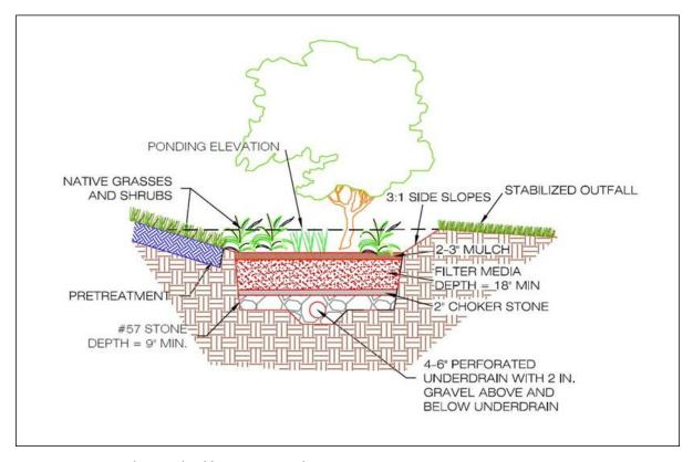
Figure 4.4. Example standard bioretention design.
